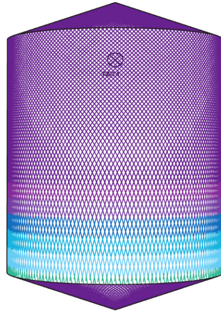
D5m H6m, Toftejorg TZ-74 Self Cleaning version, 4 x \varnothing 7 mm, 0% Time = 15.3 min., Water consumption = 4853 l
