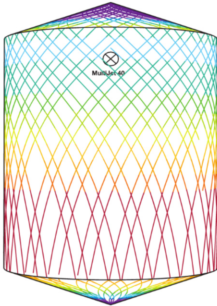
D5m H6m, Toftejorg MultiJet 40, 4 x ø6 mm, 100% Time = 4.3 min., Water consumption = 887 l
