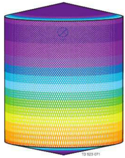
D4.6m H5.5m, Toftejorg TJ 20G, 4 x ø5.5 mm, Time = 8.3 min., Water consumption = 1612 l
